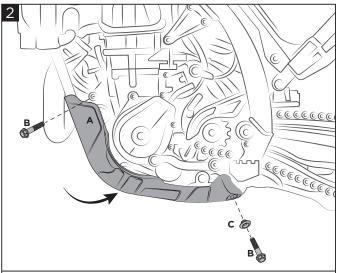
Position the Acerbis skid plate (A) and fix it using the supplied
